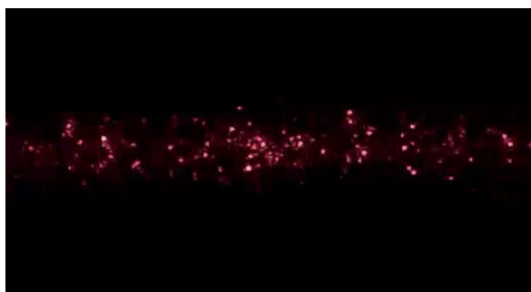
Fig. 3. Ultramicroscope field of view image of a 0.1 g/l asphaltene solution sample in toluene after adding 74 vol% heptane by titration
